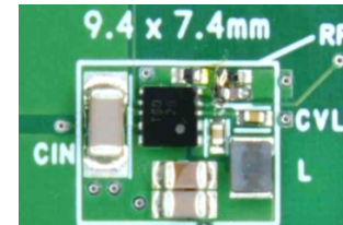
60V 300mA DC/DC : XC9702 World's smallest class of solution size 9.4mm x 7.4mm = 69.6mm 2
