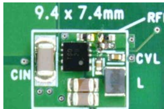
60V 300mA DC/DC : XC9702 World's smallest class solution size 9.4mm x 7.4mm = 69.6mm 2
